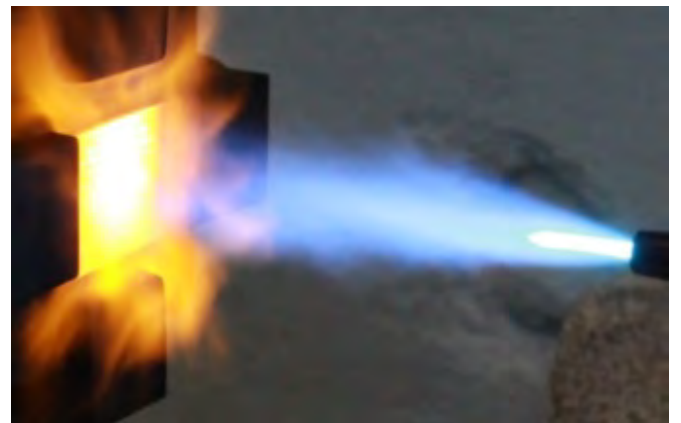
Ceramic Matrix Composite undergoing blow torch testing at 1600°C
