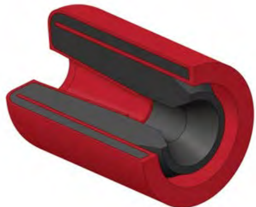
Snail charge motor that has been designed on ITP and will be built and tested in a future phase
