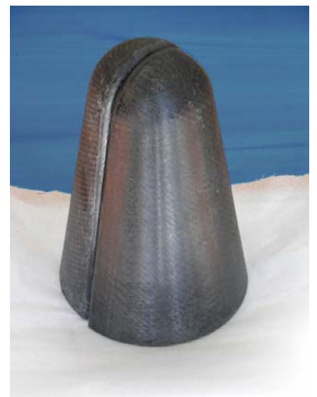
Hypersonic missile nose cone manufactured out of HVN-CMC high temperature carbon fibre
