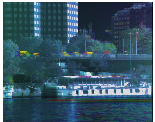
Cars travelling across a bridge in a complex urban/littoral scene, clearly separated in yellow from the background using polarisation
