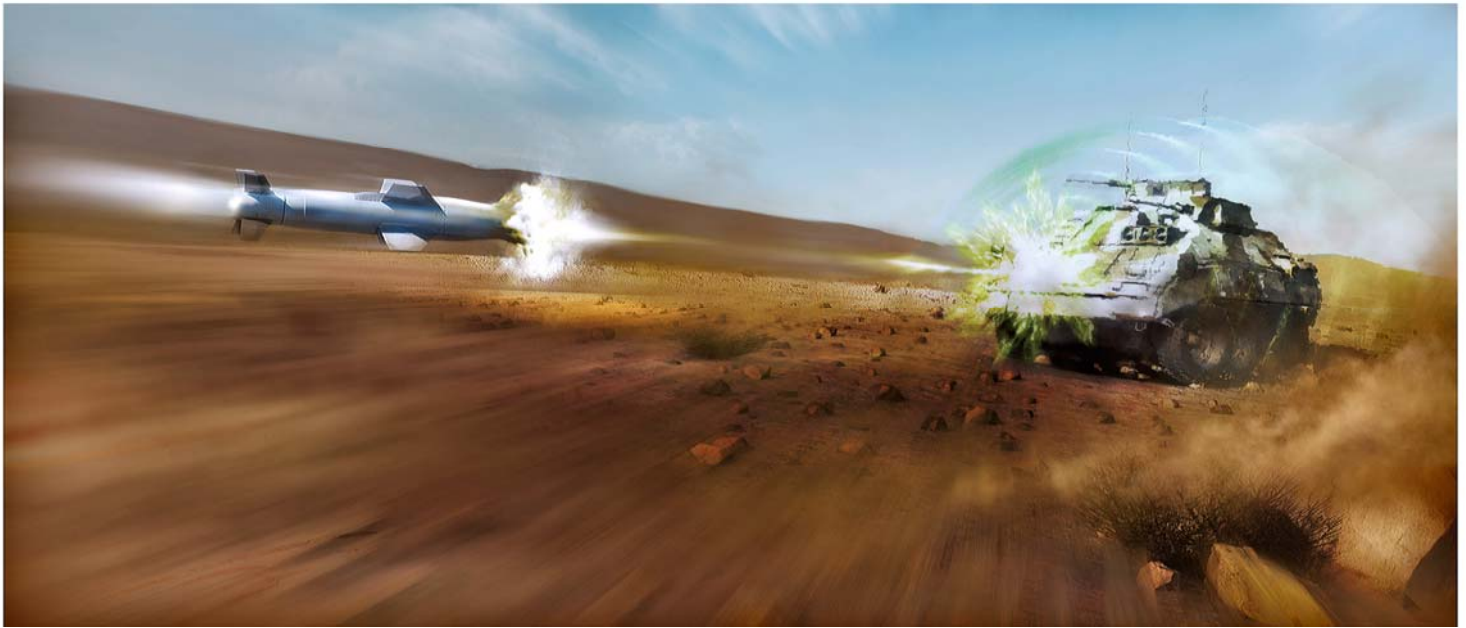
Artist's impression of a battlefield missile penetrating an armoured vehicle protected by a Defensive Aid Suite (DAS) using a long stand off warhead
